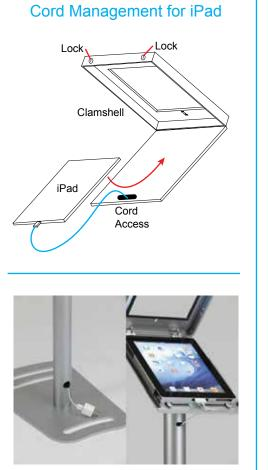
Attach iPad cord to supplied USB extension cord. Feed USB cord through top hole of post, then out bottom hole of post. Connect to power.
